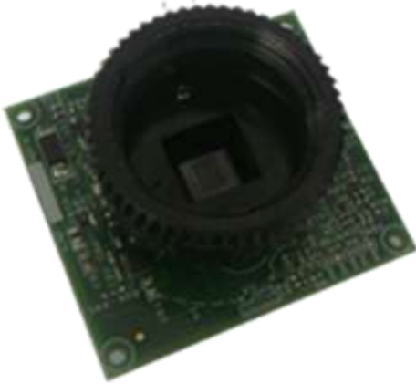
Figure1: See3CAM_10CUG - 1MP Global shutter camera with CS Mount Lens holder
