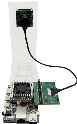
Figure 1: e-CAM50_CUCRL with Coral Development Kit
