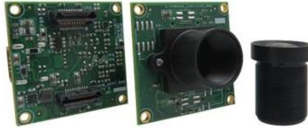
Figure 2: Conversa (See3CAM_CU38) - AR0330 Camera Module, USB 3.0 Interface Board and Lens
