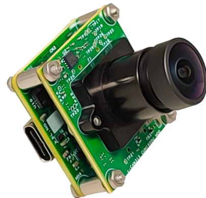
Figure 1: See3CAM_37CUGM HDR Global Shutter USB Camera (without Enclosure)
